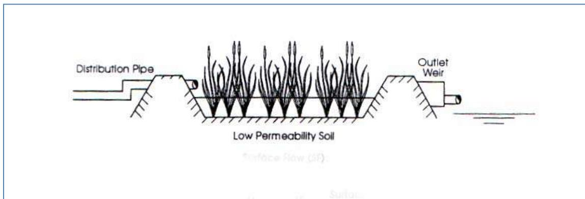
Figure 1 - Basic concept of a WTS bed
